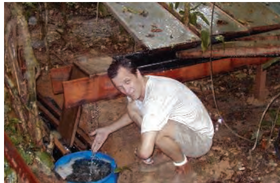
Diversion. Panels and gutters caught rain, enabling Daniel Nepstad and his team to mimic a drought.
